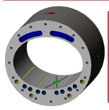
The Housing is Aluminum. A water jacket along the perimeter provides for thermal stability (blue).
