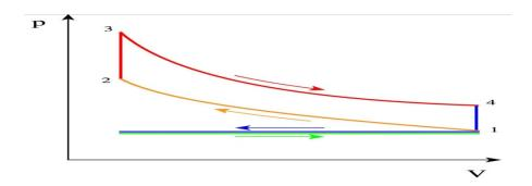
The Circle Ellipse Engine Rotor turns inside the Elliptical Housing forming four expandingcontracting regions. These directly correspond to the four-stroke Otto Cycle.
