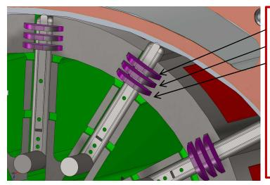
Vanes are shown installed in Rotor. Three Vane Seals surround Vanes and block combustion gases from contaminating lubrication oil, and lubrication oil from entering the combustion chamber preventing NOx pollutants.
