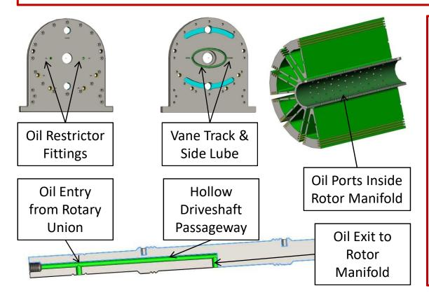
Cooling Oil enters the engine through the rotary union, passes through the hollow driveshaft, and exits into a manifold in the rotor. From there, distributed ports allow oil to flow into the rotor to lubricate the vanes, apex seals, and remove heat. A sump drain is located in the bottom of the housing to evacuate excess oil every revolution, which is defoamed, filtered, and returned.
