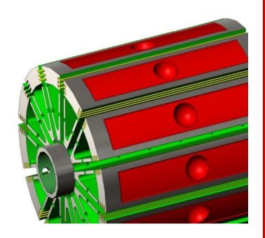
The rotor is partitioned into 12 sectors. Each sector includes slots for vanes, and multiple vane seals to isolate combustion areas from lubrication areas. In combination with the drive shaft, the rotor mass provides the fly wheel function.
